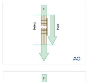
Load bearing In load-bearing fixation the plate assumes 100% of the functional loads.
